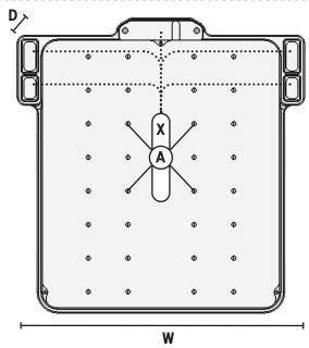
external dimensions max.: **H** = 220mm **W** = 218mm **D** = 10mm
